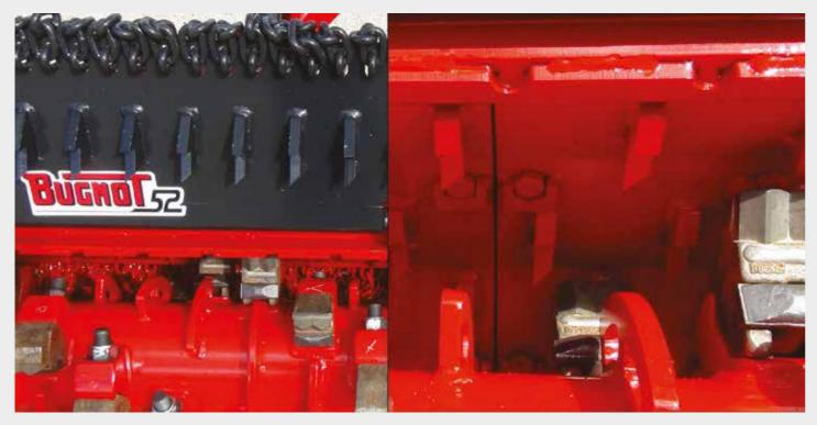
For an optimum grinding, the mulcher is fitted with counter knife shearbars at the front and above the rotor as well as on the hydraulically operated rear door ROTORS DESIGNED AND TESTED WITH AND FOR YOU STURDY LOCATING AND LOCKING OF THE HAMMERS EASY AND QUICK CHANGE OF THE WEARING PARTS
